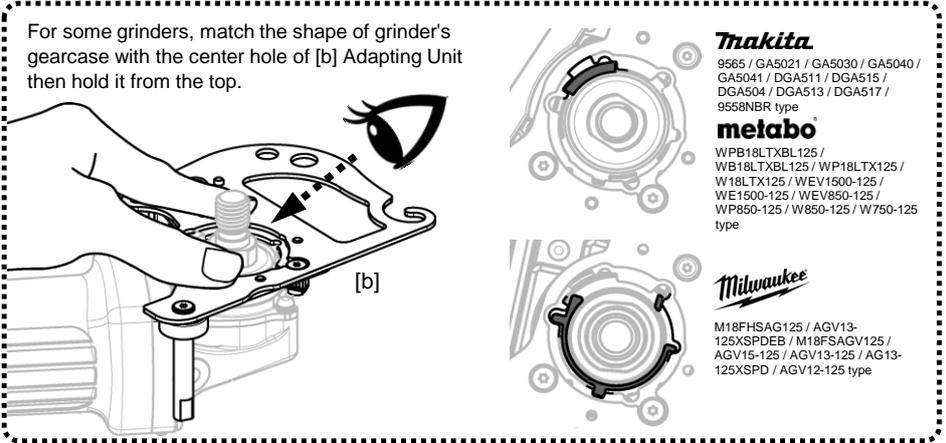
6. Keep holding [b] Adapting Unit and tighten the Bolt with [d] Wrench securely.
