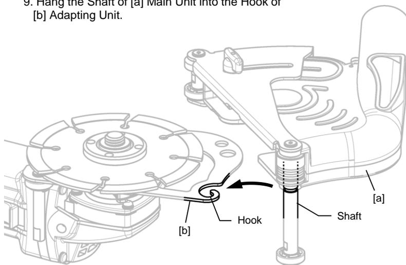
10. Rotate [a] Main Unit toward [b] Adapting Unit with Shaft as axis.
