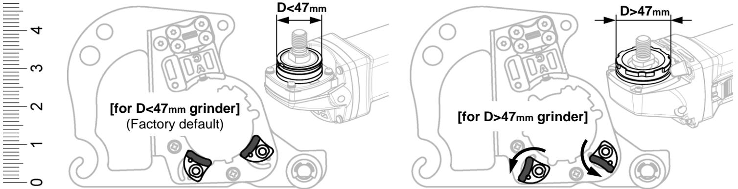
4. Place [b] Adapting Unit on gearcase of the grinder.
