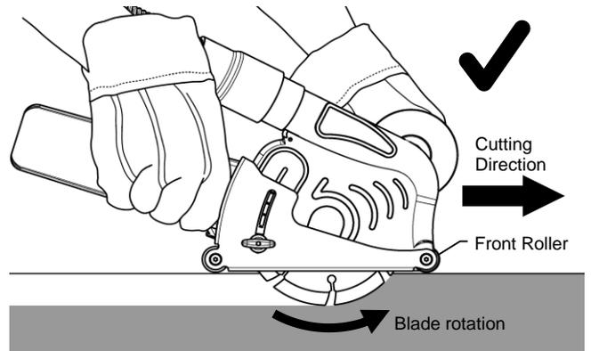
**!** DO NOT lift or move backward the angle grinder as it leads to the scattering of the Dust.
