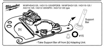
3. Switch the Lower Brackets position when the gearcase size D of the angle grinder is larger than 47mm.
