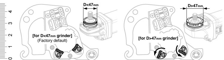
4. Place [b] Adapting Unit on gearcase of the grinder.
