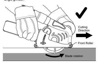
$\sum$  DO NOT lift or move backward the angle grinder as it leads to the scattering of the Dust.
