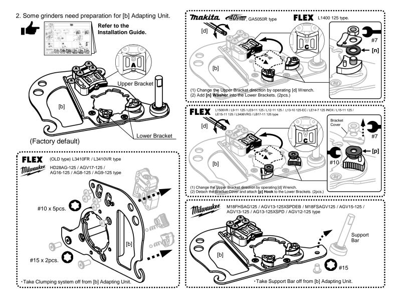
3. Switch the Lower Brackets position when the gearcase size D of the angle grinder is larger than 47mm.
