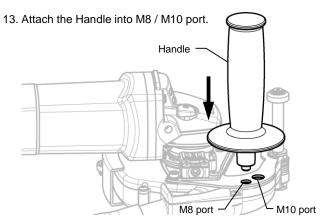
Securely hold the angle grinder and handle.
