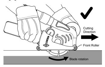
extstyle o DO NOT lift or move backward the angle grinder as it leads to the scattering of the Dust.
