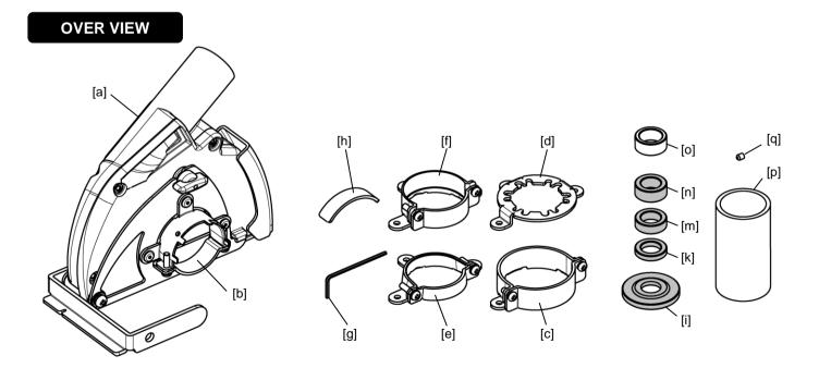
[a] Main Unit, [b] M-Connector, [c] B-Connector, [d] F-Connector, [e] H-Connector, [f] D-Connector, [g] Wrench, [h] Collar, [i] Base Flange, [k] T4.5 Spacer, [m] T7.3 Spacer, [n] T9.4 Spacer, [o] T10 x id16 Spacer, [p] Hose Adapter, [q] Set Screw.
