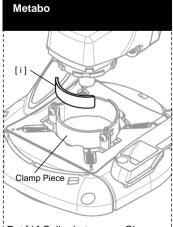
Put [ i ] Collar between a Clamp Piece and angle grinder.
