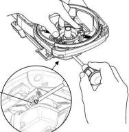
(2) Set the correct Connector and tighten the screws. (Don't forget to fit the washers)
