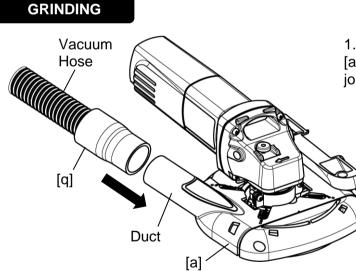
1. Securely connect the Vacuum Hose to the port of [a] Main Unit, using [q] Hose Adapter or other suitable joint between the port and Vacuum Hose.
