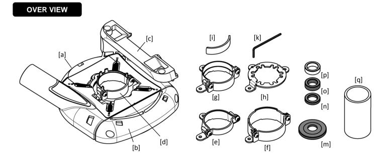
[a] Main Unit, [b] Sub Cover, [c] Half Cover, [d] M-Connector, [e] H-Connector, [f] B-Connector, [g] D-Connector, [h] F-Connector, [i] Collar, [k] Wrench, [m] Base Flange, [n] T4.5 Spacer, [o] T7.3 Spacer, [p] T7.3 x iD16 Spacer, [q] Hose Adapter.
